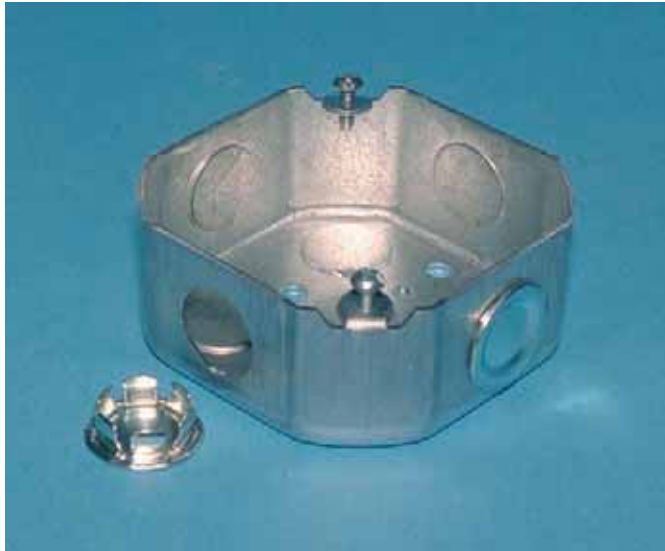
Figure 9-1 Section 110.12(A) requires unused cable or raceway openings in electrical boxes to be effectively closed.
