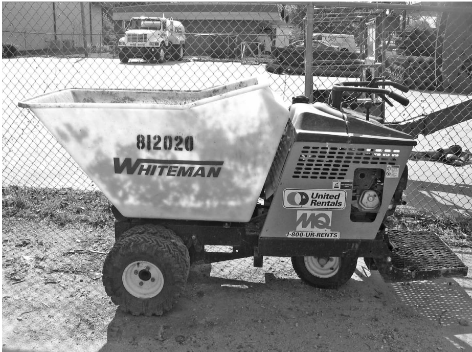
Figure 1-1 Motorized wheelbarrows (sometimes called wheelbarrels) can be a great time-saving tool because they can carry heavy loads with ease.
