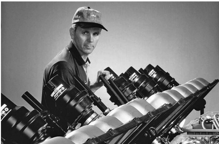
Figure 1-2 Here a worker installs garbage disposals in an assembly line fashion. This will be a great time-saver when compared to doing it on the jobsite. Courtesy of Marlin Mechanical Corporation, Phoenix, AZ.
